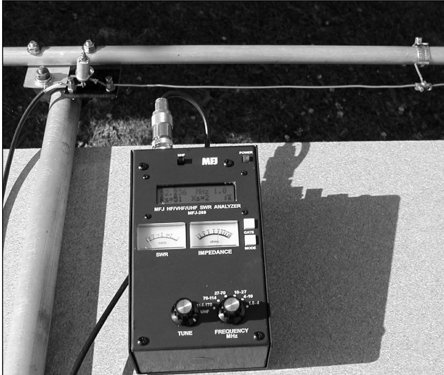
Fig 14.31: Simplified Gamma match by G3LDO uses hard drawn copper wire as the gamma rod. Connection of the gamma rod to the antenna element is achieved using a hose clamp. A Philips capacitor is used as a reactance correction capacitor, which can be replaced with a fixed mica capacitor of the correct value (see text) once the adjustments are complete.
