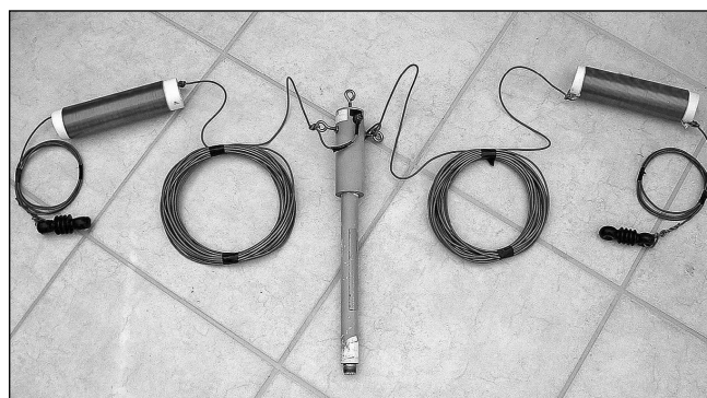
Fig 15.12: The antenna components of the 80 / 40m loaded dipole, together with a commercial Ferromagnetics current balun at its feedpoint
