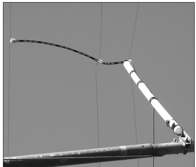
Fig 15.79: Detail of the multiband quad feed arrangement. A plastic tube is fixed to the mast to provide support for coax feeder. Connector blocks were originally used for connections to the elements but this has since been modified - see text
