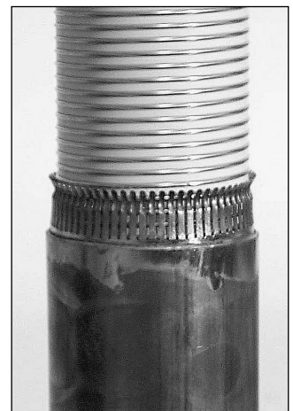
Fig 15.92: Detail of the tuning section of the 'screwdriver' antenna, which shows the coil and fingers that short the turns as it emerges. This photo, courtesy of Waters and Stanton plc, is of the WBB-3 derivative
