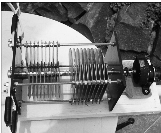
Fig 15.60: Example of one of GW3JPT's home made capacitors
