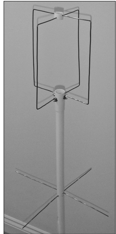
Fig 16.92: K5OE Eggbeater II without weatherproofing
