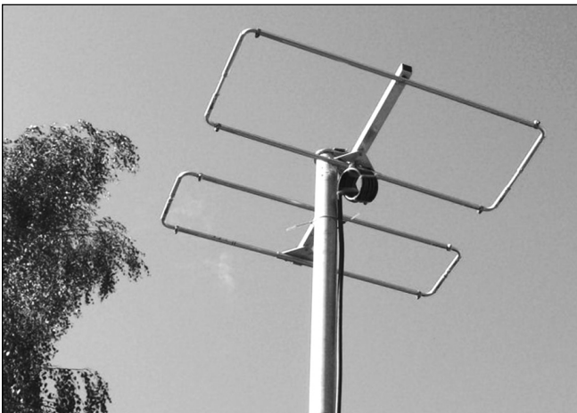
Fig 16.20: The 2m version of the Super Moxon is just 30" x 25"
