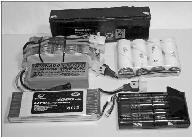
Fig 18.38: Selection of batteries for outdoor operations. Clockwise from the bottom left: 4.0 Ah 3S LiPo pack (265g); 2.2 Ah 4S LiPo pack (242g); 3.3Ah 13.2V NiMH Sub-C pack (796g); 2.2Ah 12V SLA battery (824g); 2.3Ah 4S LiFePO4 pack (314g); 2.6Ah 9.6V NiMH AA cell pack (258g). It is no coincidence that of the six batteries shown, half are based on Lithium. For robustness and ease of use, NiMH is still to be preferred, but for the ultimate in performance, LiPo is the clear favourite. The two packs at the front are intended for use with the FT817 - indeed the one to the right uses the FT817's AA cell carrier. The voltage of the 3S LiPo is ideal for the FT-817 and this pack will power the rig for a multi-summit expedition without needing to be recharged. The remaining packs are for use with mobile transceivers such as the FT-857 which can be powered directly from all but the 4S LiPo pack. Here, the 100% SOC voltage exceeds the maximum voltage specified by most equipment manufacturers and so the diode dropper described earlier in this section should be used.
