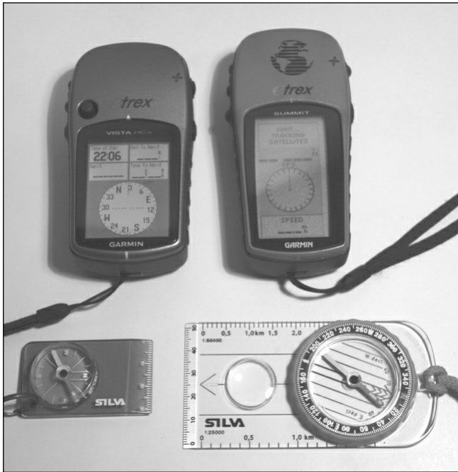
Fig 18.3: A selection of navigation tools: The newer Etrex Vista HCx on the left has a colour screen and higher sensitivity receiver than the older Summit on the right. The small Silva compass below it may be adequate as a backup. The Silva Ranger 3 on the right is preferable
