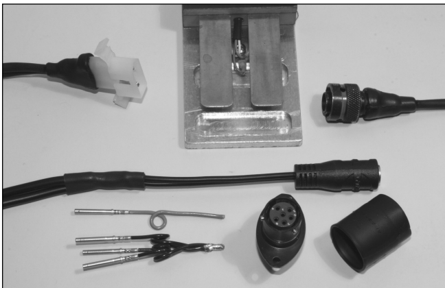
Fig 18.2: Strain relief applied to control cables. 1) Top centre shows how the cable into the centre of this paddle key is trapped and held by the Tufnol block. Each connection has a small length of Kynar heatshrink sleeving covering the solder joints. 2) Top left and right are examples of heatshrink boots being used to protect the cable exits from connectors. 3) A headphone splitter made from three moulded cables. The splice contains sleeved, Kynar-covered joints with repair loops and there is a heatshrink covering for overall protection of the split. 4) Bottom left is an example of 'repair loops' - a small loop allowing the wire to be stretched slightly without damage. Note the crimped pins. 5) Deutsch Autosport connector and Raychem boot prior to shrinking. The connector is the intended housing for the crimped pins to their left
