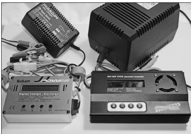
Fig 18.39: A selection of intelligent battery chargers. The two chargers at the rear are mains-powered units specifically for SLA batteries. The large unit to the right is a Yuasa YCP4A12 three-stage charger delivering 4A. The Mascot plugtop unit to the left is for smaller batteries and charges at a maximum of 0.5A. On these units, LEDs indicate the status while charging. The two 12V-powered chargers at the front will cope with a range of chemistries. Both will cope with Lithium, NiMH and NiCD batteries however the unit to the right will also charge SLA batteries and all three types of Lithium batteries. Note the ferrite chokes that have been added to the leads on the Kokam unit to reduce spurious emissions. Most chargers of this type have a small alphanumeric display which is essential for their setting up and operation.
