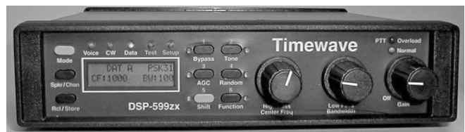
Fig 19.17: The Timewave DSP-599zx is an add-on DSP filter which can improve CW reception
