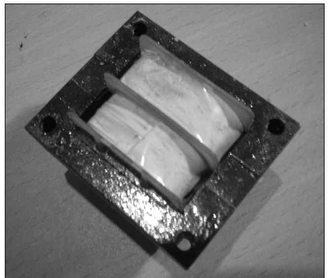
Fig 2.21: A transformer with the primary and secondary wound separately, with an insulated divider
