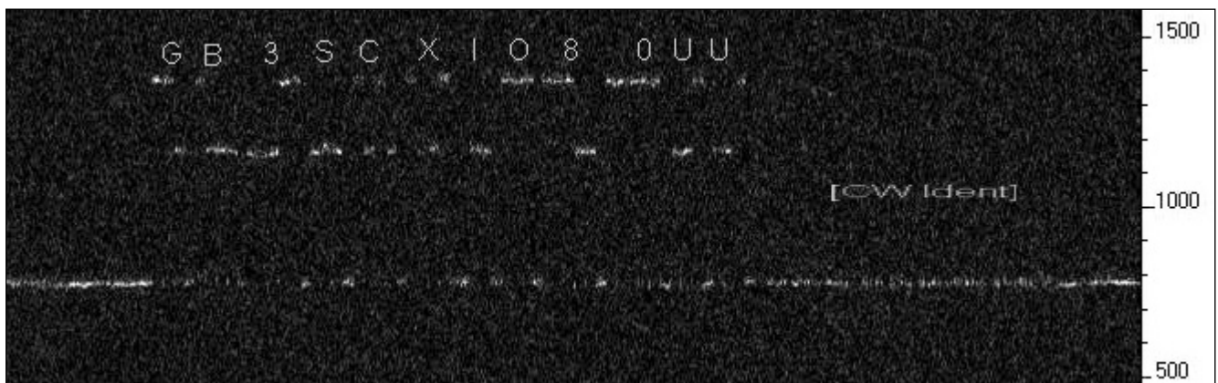
Fig 20.12: Weak signal DFCWi reception of the GB3SCX beacon on 10GHz (the callsign letters have been manually added to the picture for clarity). Dashes are on the top line, dots on the middle and the idle state on the bottom.
