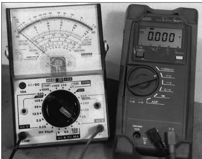
Fig 24.1: Typical analogue and digital multimeters
