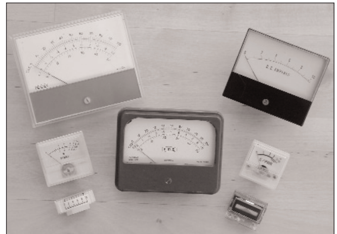
Fig 24.2: Various moving-coil and moving-iron meters
