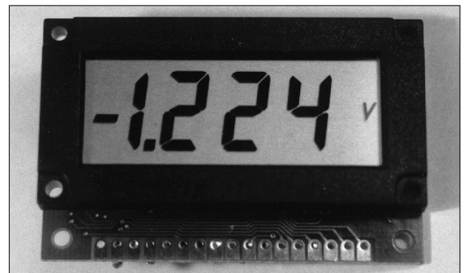
Fig 24.17: A typical digital panel meter
