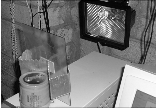
Fig 25.36: Simple exposure unit using 500W security lamp
