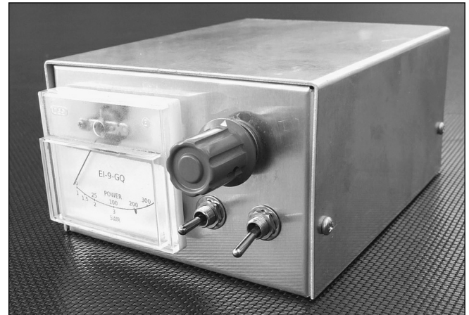
Fig 25.6: SWR meter enclosure using the score and bend method
