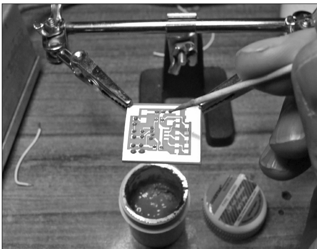
Fig 25.45: Applying the solder paste to one of the PCBs using a cocktail stick
