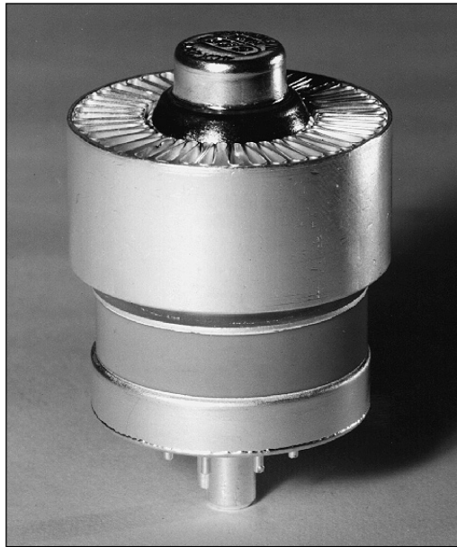
Fig 3.86: 4CX250B showing its air- cooled vanes
