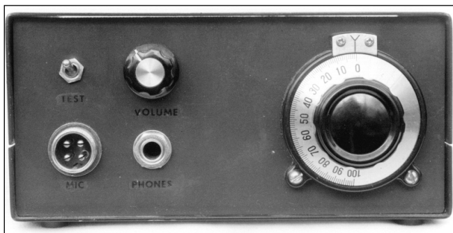
Fig 7.36: Front view of G3TXQ QRP transceiver. On this prototype the TUNE switch is labelled TEST
