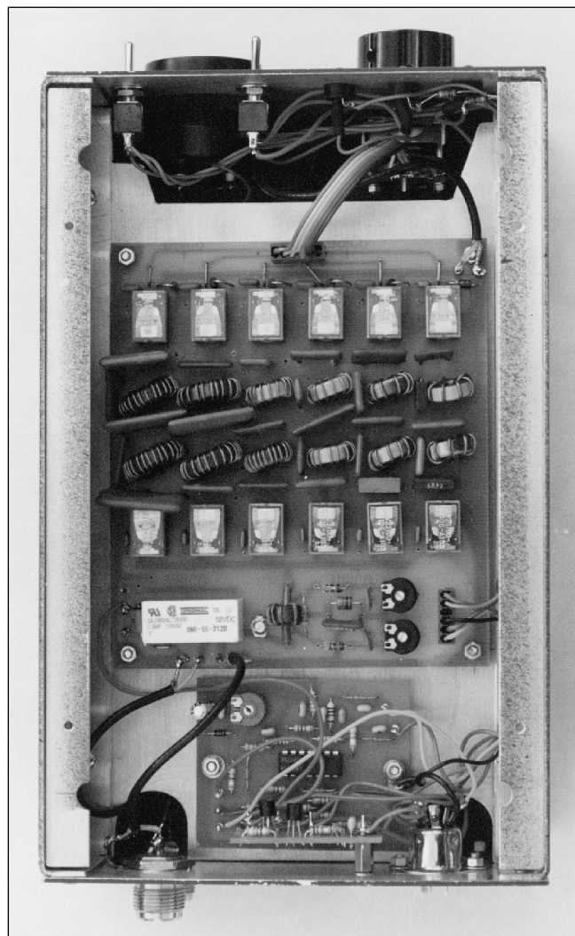
Fig 7.62: Low-pass filter and ALC circuits
