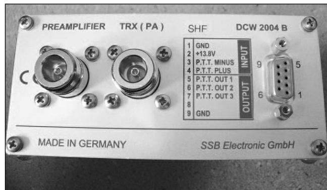
Fig 9.64: Rear panel view of the DCW2004B SHF sequencer showing the N connectors and 9 pin D connector used for powering and interconnections to the transceiver and power amplifier (if used). The non-SHF version looks similar
