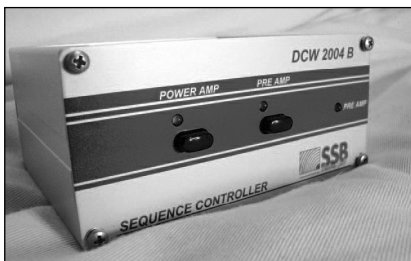
Fig 9.63: DCW2004B sequencer, Note the preamplifier and power amplifier enable switches and indicator LEDs
