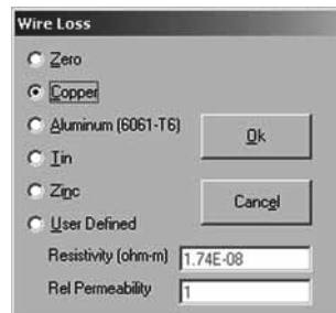
Fig 4.11: Wire Loss window for the G5RV.
