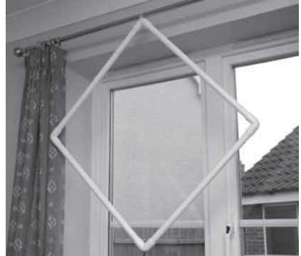
This tiny 21in square antenna made out of PVC tubing and wire made an easy contact into the Netherlands with just 5W.
