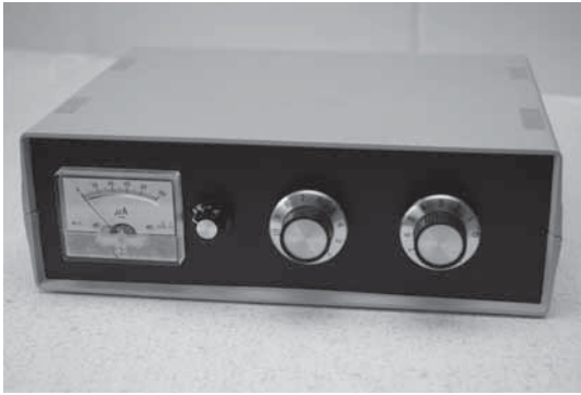
The tuner consists of just two variable capacitors. The meter is optional.
