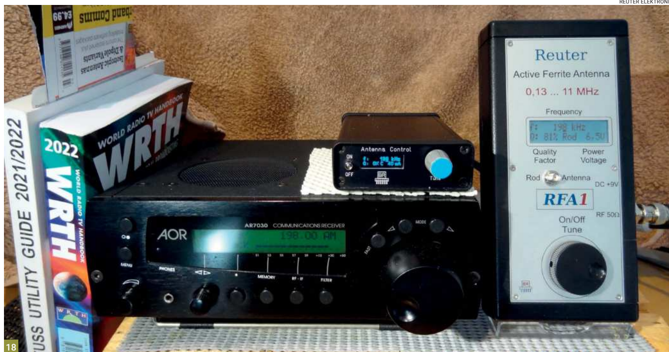
Fig. 18: The Reuter Elektronik RFA1A Active Ferrite Antenna & RWS4 Aerial/ Remote Control Unit.
