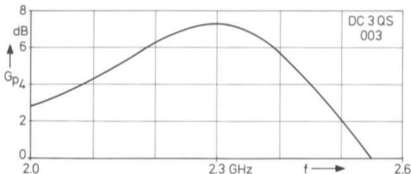
Fig. 5: The described amplifier can be used without tuning from 2.2 to 2.4 GHz
