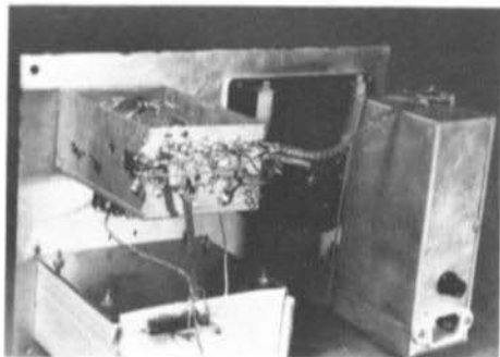
Fig. 11: Inside are 3 screened modules and a meter
