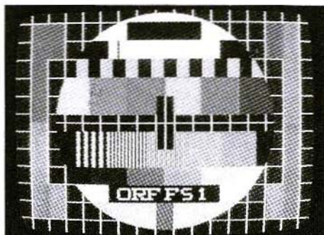
C / N = 40 dB: Picture noise-free (in commercial practice a picture is considered noise-free at 60 dB)
