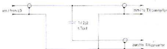
Fig. 16: A simple method of splitting the oscillator signal to feed both transmit and receive mixers.
