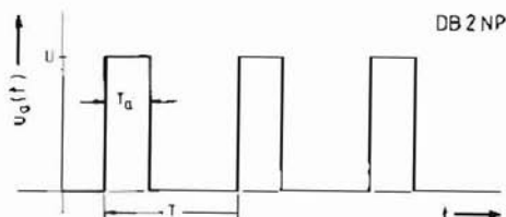
Fig. 2: Typical output signal of a monostable being triggered at a frequency f = 1/T
