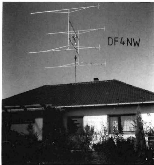
Fig. 7: The author's 4 x 17-el. Yagi, EME array.
