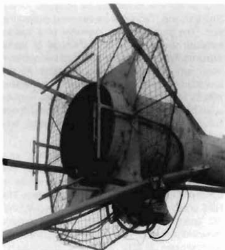
Fig. 2: Feed arrangements for 23 cm (circular) and 70 cm (H or V switchable)
