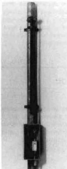
Fig. 8: The pre-amplifier/ relay unit from fig. 5 affixed to a coaxial matching trans- former
