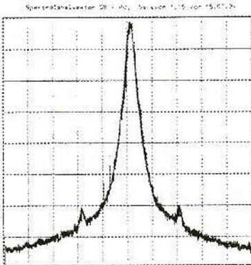
**Fig.1: Previous Spectrum Analyser LO with powerful Noise Bar**
