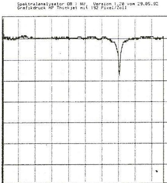
**Test Object:** S6 Notch filter
