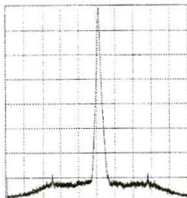
Fig.10: Smaller Noise Base, Divider Chain - CA3199 & SP8695
