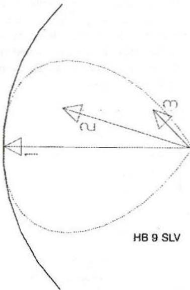
Fig.8: Example of Excitation of a Parabolic-type Reflector at various Angles:
