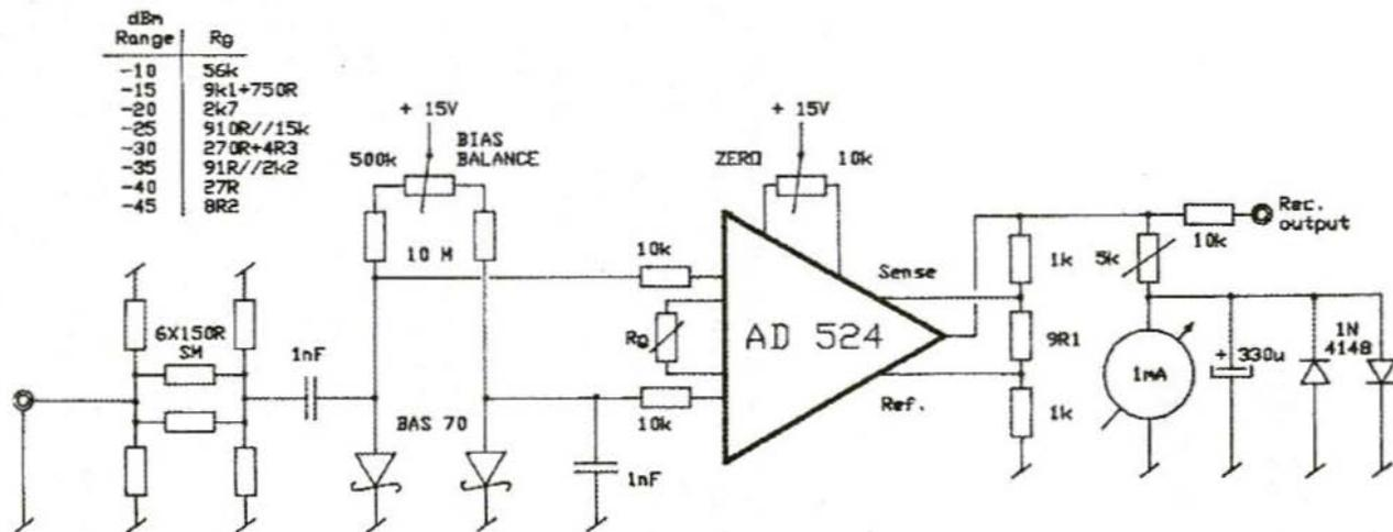
Fig.1: Circuit Diagram and Component Layout for the Power meter
