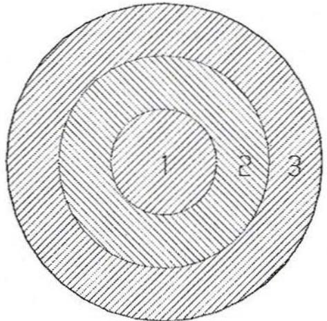
Fig.9: Area 1 corresponds to only 10% of the Exciter radiation. By contrast, Area 3 corresponds to half the total Area, but receives only 10% of the HF
