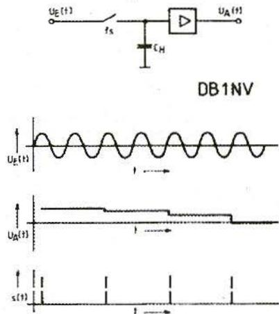
Fig.6: Structure and Operation of a Sampling Phase Discriminator
