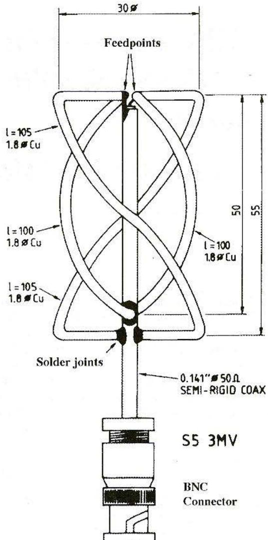
Fig.1: The Quadrifilar Backfire Antenna with Right-Hand Circular Polarisation
