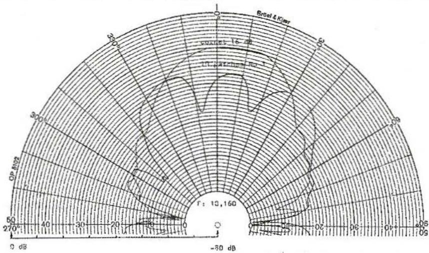
HB 9 SLV Antenne 10 patches No 1 F: 10,160 GHz d: 1 m. Ech. log. 80 dB S: 6 dB
