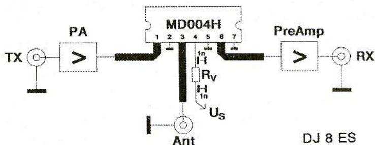
Fig. 2: Switching the MD004H Hybrid Antenna Switch Module
