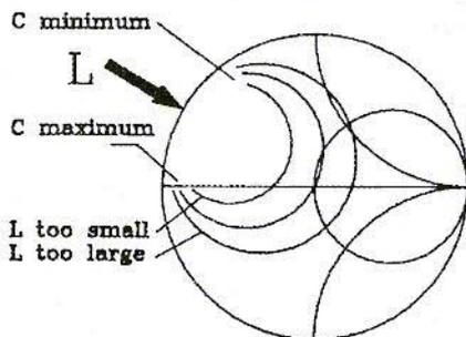
Fig.3: Effects on the Reflection Coefficient from Tuning and from varying the value of the Small Inductor
