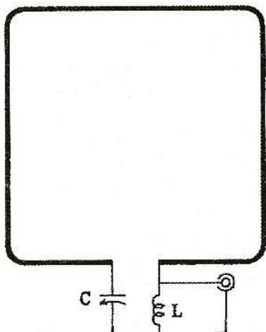
Fig.2: The improved version with an Inductive Divider
