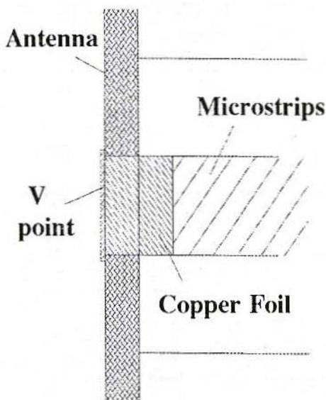
Fig.5a: Antenna powered through Strip
