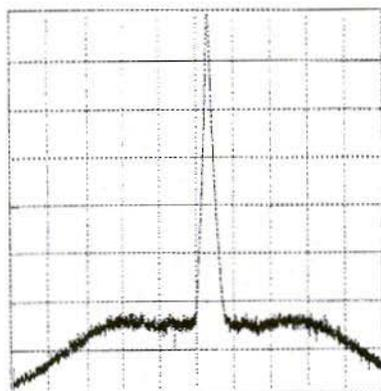
Fig.9: Noise Base using SP 8716 Divider
