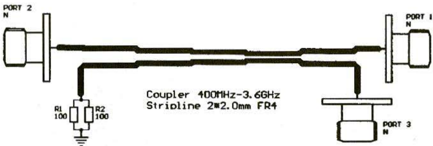
Fig.2: Wiring Diagram of Asymmetrical Stripline Coupler
