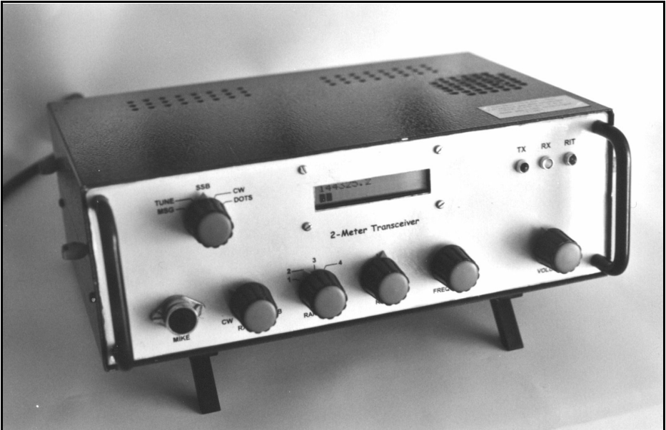
Fig 2 : Photograph of the completed 2m direct conversion transceiver.
