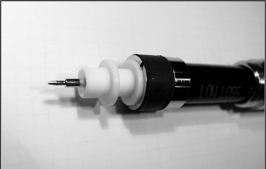
Fig 3 : The tefflon inner part of a plug designed for use with ECOFLEX 15 cable. It is specially designed to reduce impedance jumps in the plug body.
