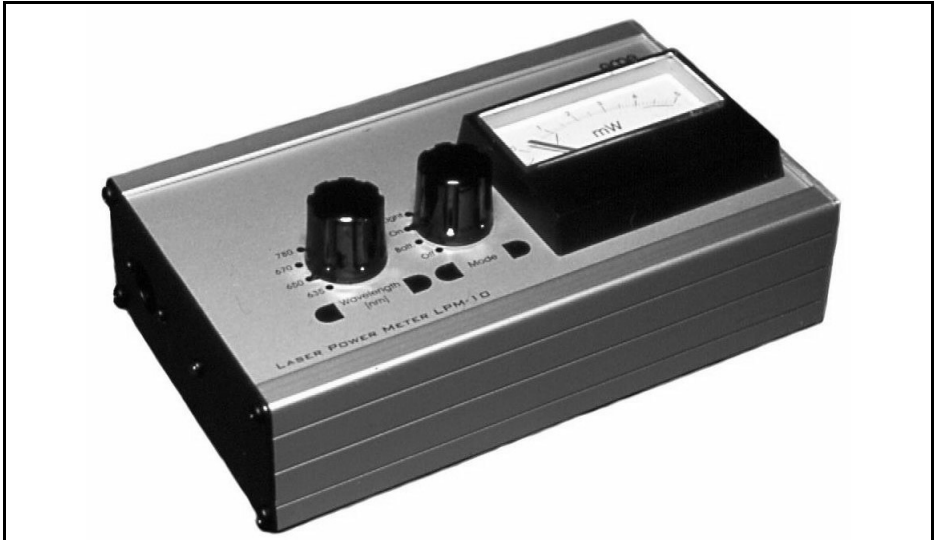
Fig 10 : The prototype of the LPM-10 laser output meter.
