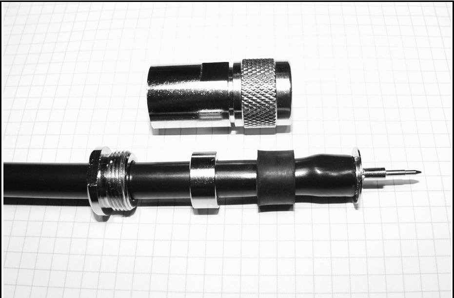
Fig 1 : N type plug with extended body and improved clamp. This plug was specifically designed for use with AIRCOM plus cable.
