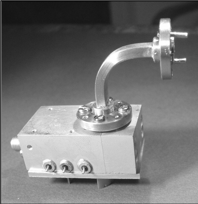
Fig 3: Side view of the completed transmitter showing the output feed and DC supply via feed through capacitors.
