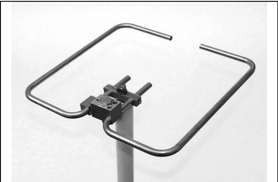
Fig 1: Photograph of the 2m H O Loop antenna from M 2 -Inc.
