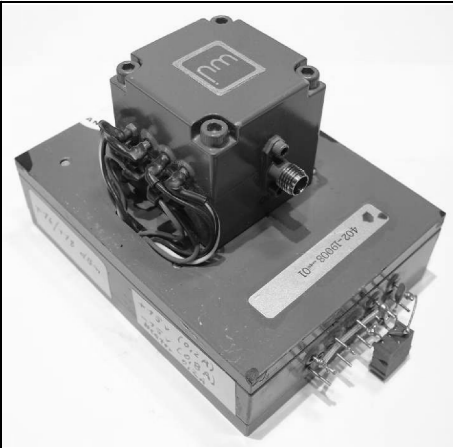
Fig 14: A second example of a YIG oscillator with a built in driver.
