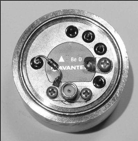
Fig 7: A YIG oscillator with no FM mode.
