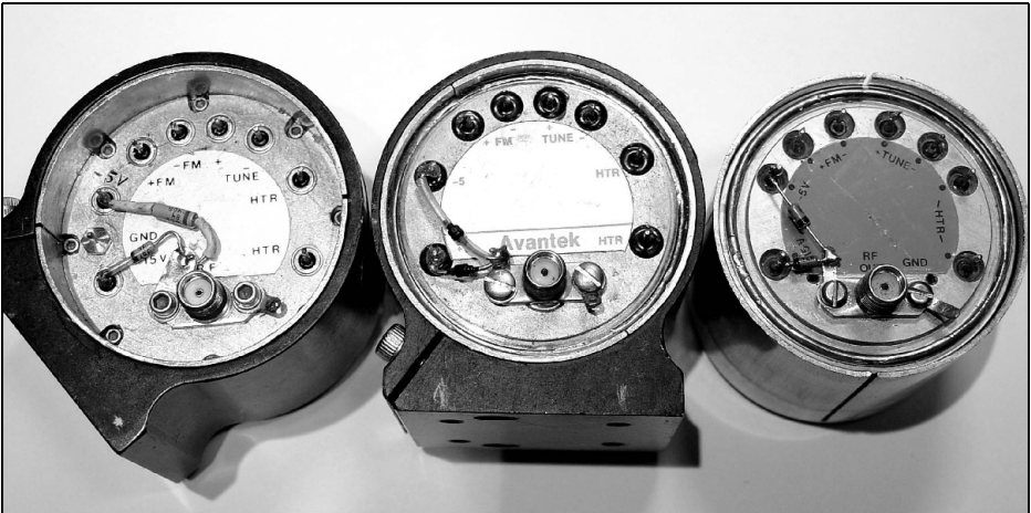
Fig 3 Examples of YIG oscillators with operating voltages of +15v and -5v.
