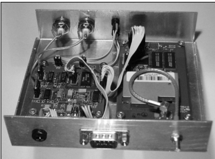
Fig 9: Rear view of the completed GPS controlled frequency standard.
