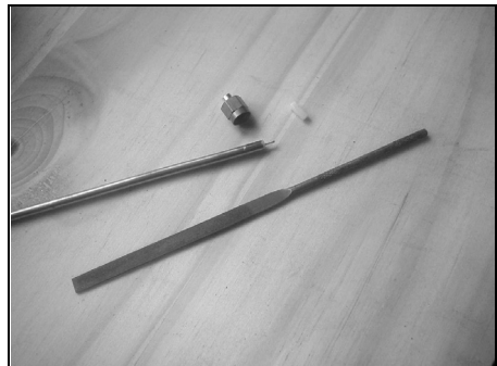
Fig 4: UT-141 cable prepared for fitting the SMA male connector. The warding file and PTFE insulator are shown.
