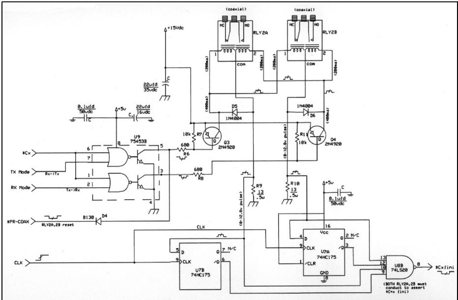
**Fig 5: T-R sequencer dual pulse latching coaxial relay.**
