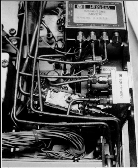
**Fig 3: The MMIC amplifier module that follows after the new mixer; built into a tinplate housing.**
