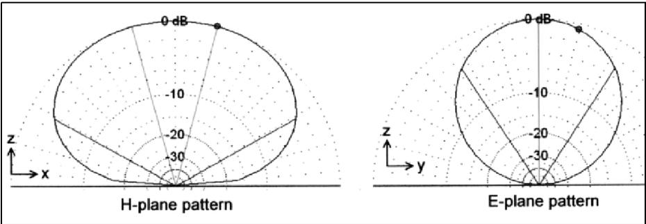
**Fig 6: Radiation patterns for a full-wave dipole over a conductor plane.**
