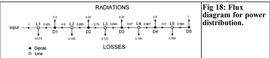
**Fig 18: Flux diagram for power distribution.**
