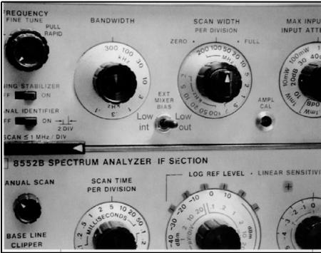
**Fig. 5: Arrangement of the new switch on the front panel.**
