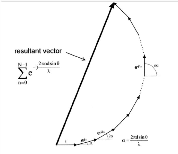
**Fig 3: Geometric interpretation of the array manifold.**
