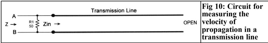
**Fig 10: Circuit for measuring the velocity of propagation in a transmission line**
