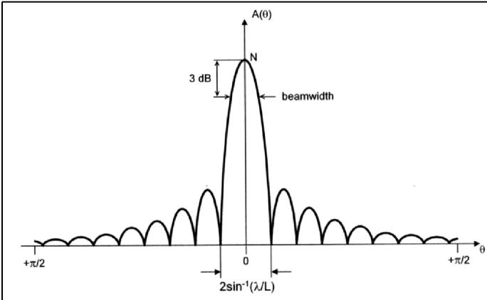
**Fig 4: Absolute value of manifold as a function of.**
