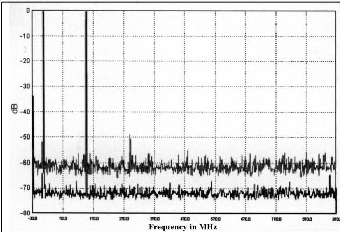
**Fig 11:** These curves document the difference between the original mixer and the new mixer; the conditions are identical for both curves.
