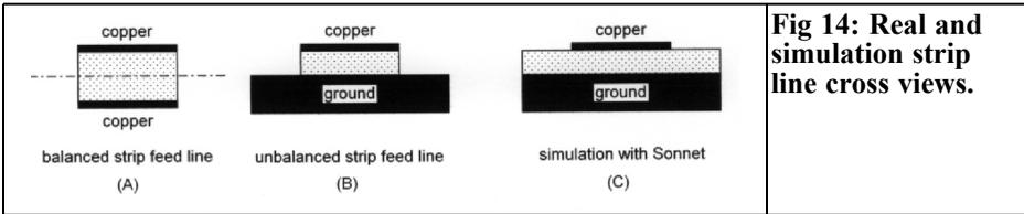
**Fig 14: Real and simulation strip line cross views.**
