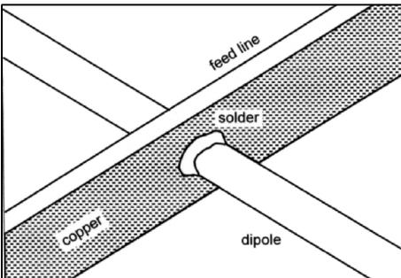
**Fig 9: Detail of the dipole soldered to the feed line.**
