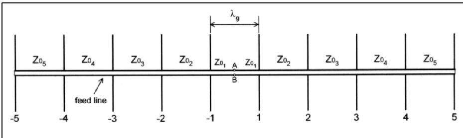
**Fig 19: Feed line with impedance optimised at each section.**
