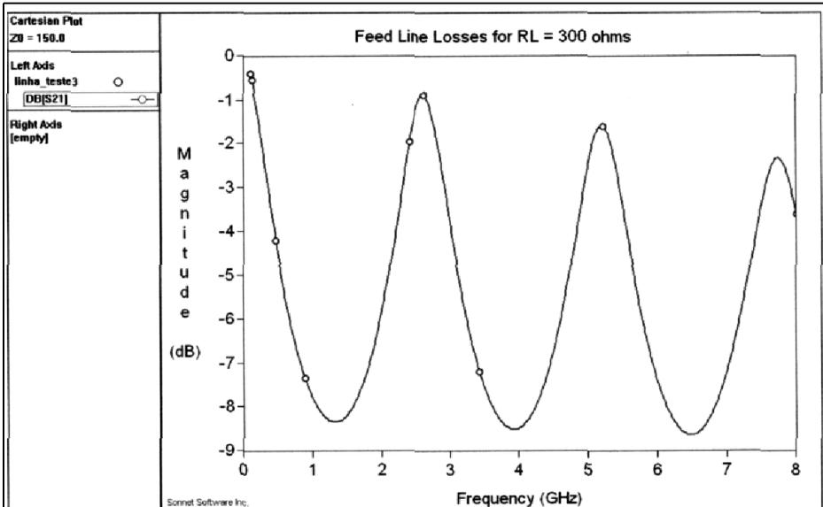
Fig 16: Transmission loss simulated for a 3mm wide, 30mm long, FR-4 strip line with RL equal to 300Ω.
