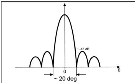
**Fig 21: Measured radiation pattern.**
