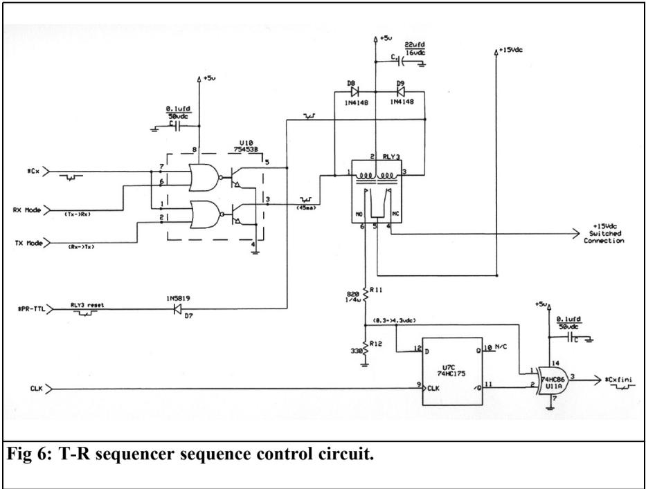
**Fig 6: T-R sequencer sequence control circuit.**
