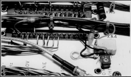
**Fig 10: The arrangement of a relay and a potentiometer for adjustment of the level in the IF port is in the right lower half. Also see the block diagram in Fig 1.**
