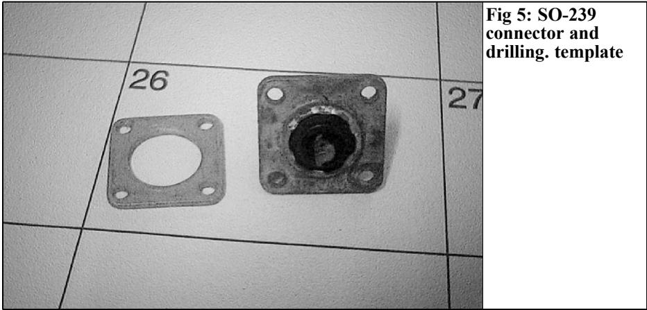
onto the panel in the required position and then use the holes to spot through with a drill bit to leave witness mark where the holes need to be drilled.
