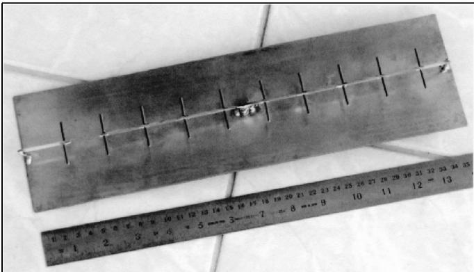
**Fig 23: Picture of the prototype antenna array.**
