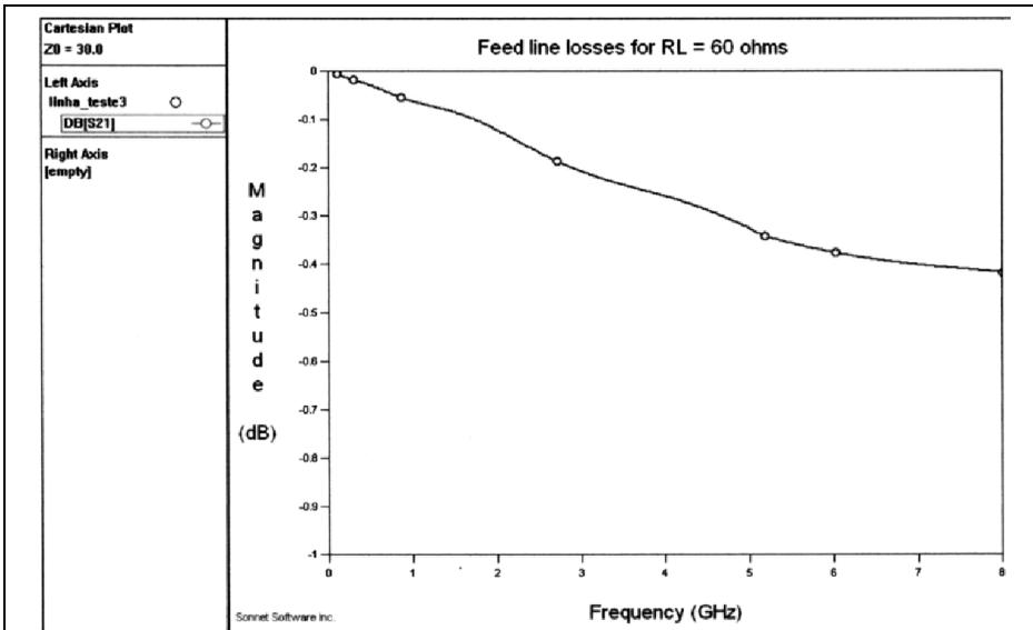
Fig 17: Transmission loss simulated for a 3mm wide, 30mm long, FR-4 strip line with RL equal to 60Ω.
