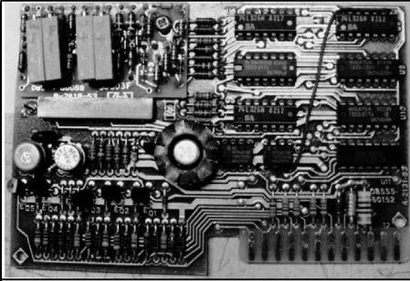
**Fig 9: A new connection is made on the front of the relay PCB.**
