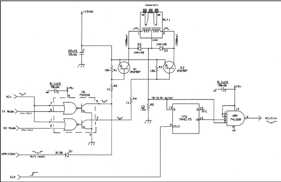
Fig 4: T-R sequencer single pulse latching coaxial relay.
