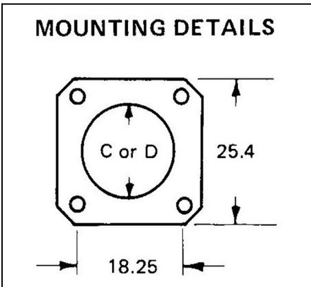
Fig 1: Dimensions for the mounting holes for the N and UHF connector.
