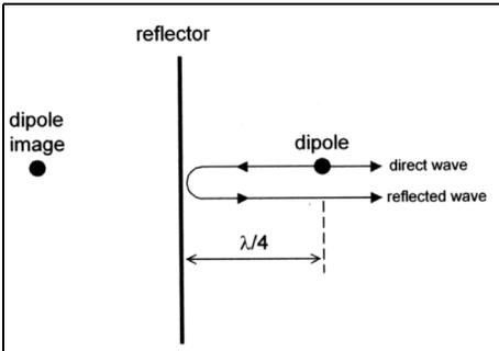
**Fig 5: Wave reflection by the reflector.**
