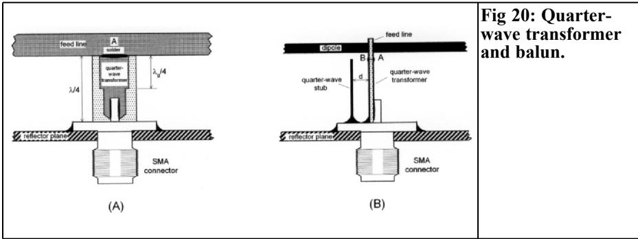
**Fig 20: Quarter-wave transformer and balun.**
