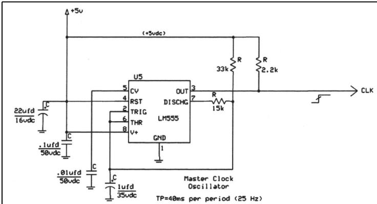
**Fig 3: T-R sequencer clock oscillator.**
