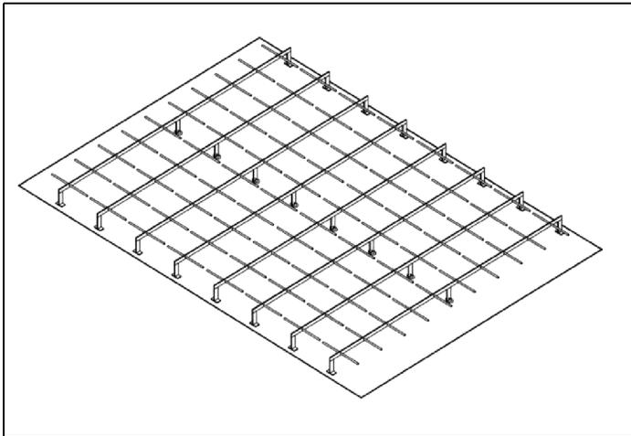
**Fig 24: A two-dimension array with 10 x 6 dipoles.**
