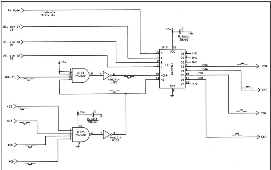
**Fig 11: T-R sequencer solid state sequencer control.**
