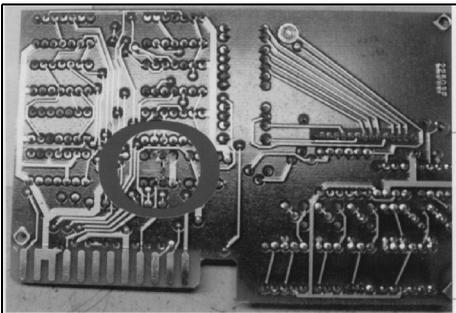
**Fig 8: A connection is isolated on the back of the relay PCB.**
