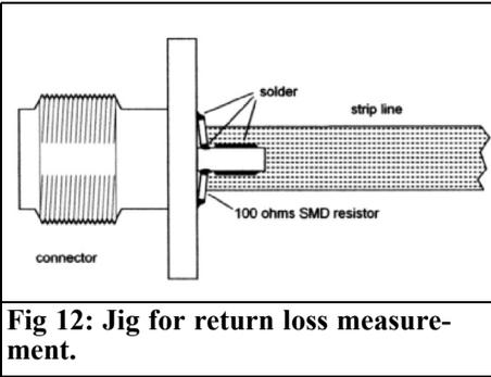
**Fig 12: Jig for return loss measurement.**
