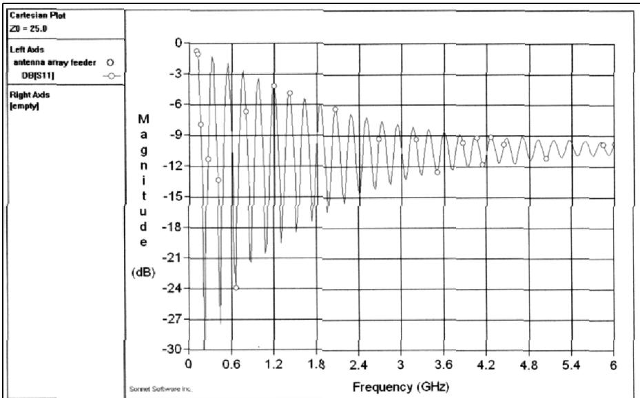
**Fig 11: Return loss of a 3mm wide and 355mm long FR-4 strip line.**
