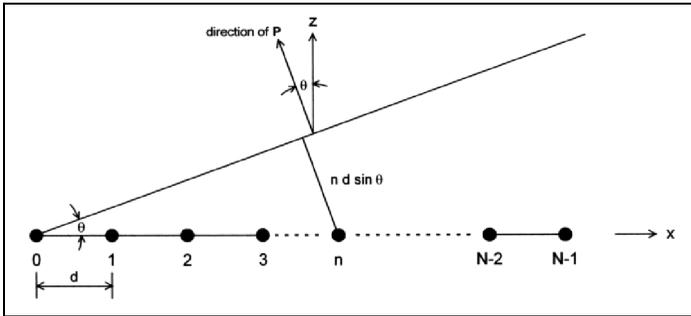
**Fig 2: Linear array with N elements.**
