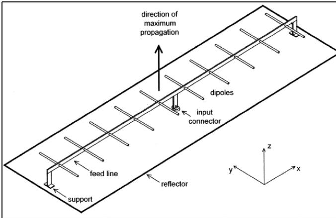
**Fig 1: Linear array with 10 dipoles and a reflector.**
