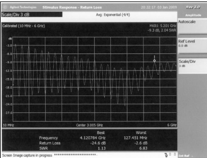
**Fig 13: Measured Return Loss of a 3mm wide and 355mm long FR-4 strip line.**
