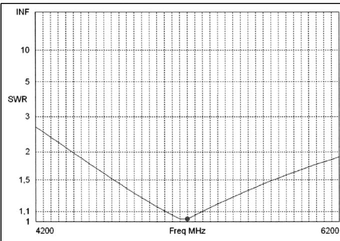
**Fig 7: SWR of a single dipole for a reference impedance of  $300\Omega$ .**
