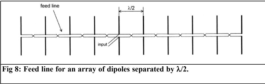
**Fig 8: Feed line for an array of dipoles separated by  $\lambda/2$ .**
