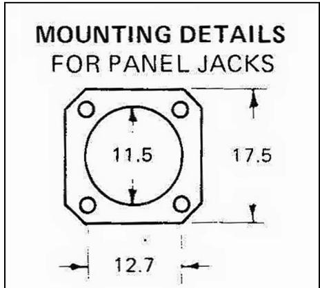
Fig 2: BNC 4-hole connector details.
