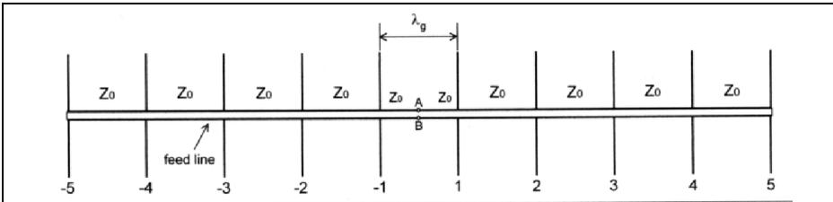
**Fig 15: Feed line with uniform impedance.**
