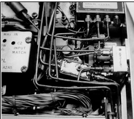
**Fig 7: All RF connections are made using semi rigid coax with SMA plugs.**
