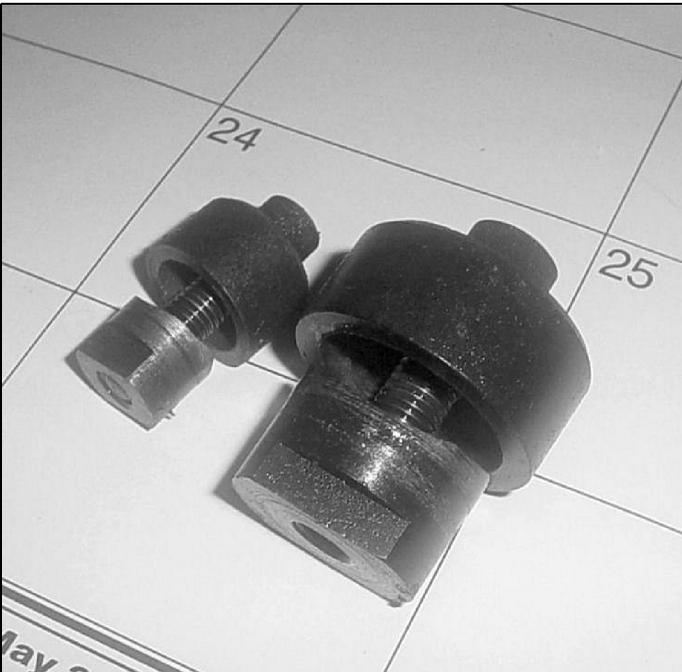
**Fig 4: Chassis punches.**
