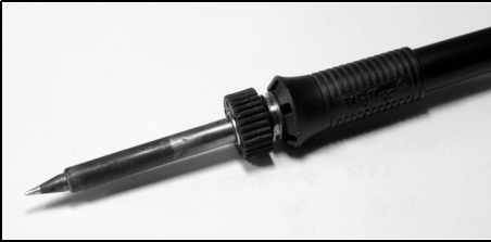
Fig 7: A WSP80 soldering iron from a Weller WS 81 soldering station. This is very suitable.
