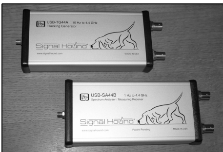
Fig 1: The SA44B spectrum analyser (front) and TG44 tracking generator.
