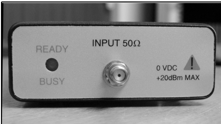
Fig 2: Front of SA44B analyser, The front of the TG44 tracking generator is similar.
