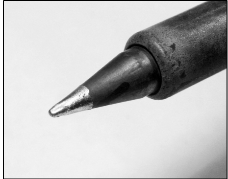
Fig 8: A 0.8mm LTH bit from a Weller WS 81 soldering station. This is very suitable.
