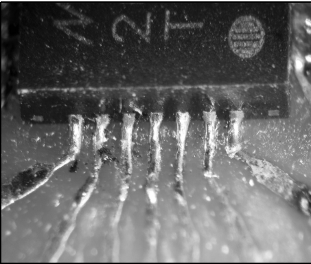
Fig 15: View of a 0.5mm IC solder using this technique on a poor PCB.
