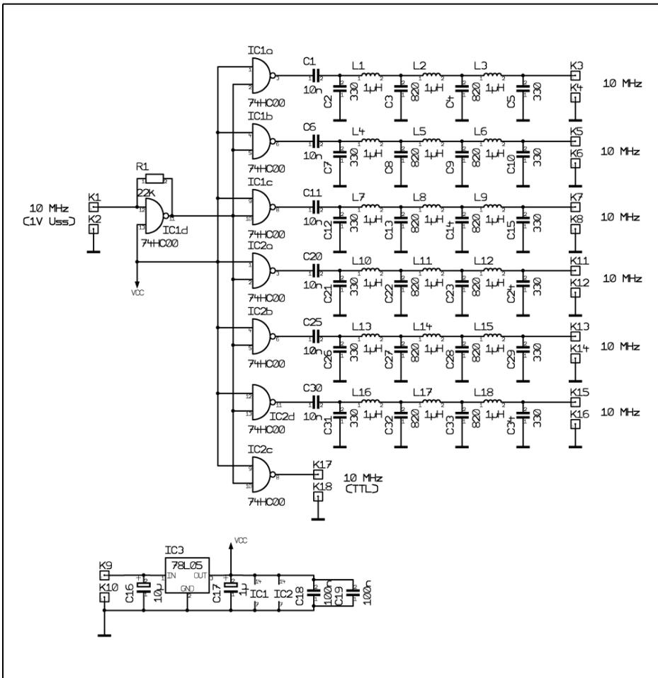
**Fig 8: Circuit diagram of the additional module for multiple 10MHz outputs.**
