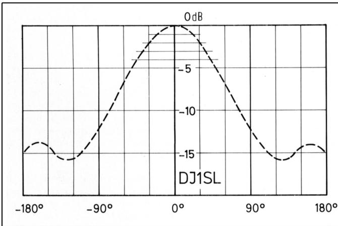
**Fig 5: Radiation diagram (E plane) of the tubular radiator.**
