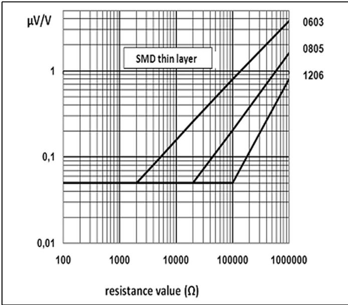
**Fig 5: Excess noise of SMD thin layer resistor.**
