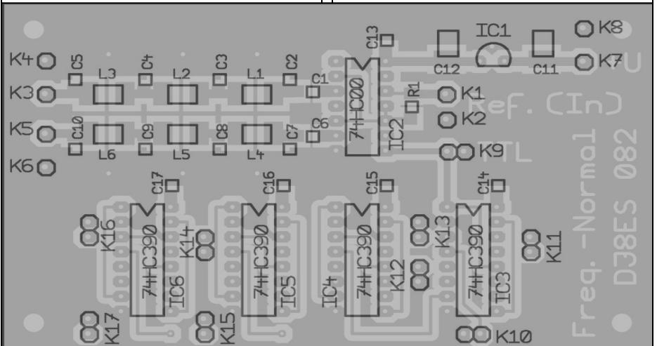
Fig 6: Component layout for the driver module.
