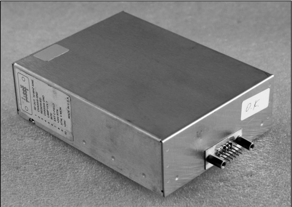
**Fig 1: The LPRO-101 Rubidium Frequency Standard module.**
