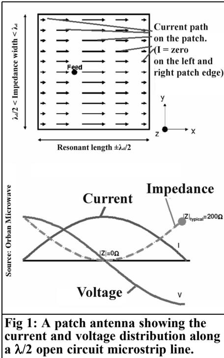
sponding to the resonant frequency produces the current and voltage distribution shown in Fig 1 (the feed point is on the symmetry axis of the patch).
