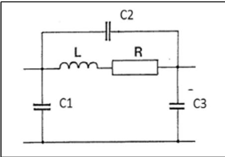
**Fig 7: High frequency equivalent circuit of a resistor.**
