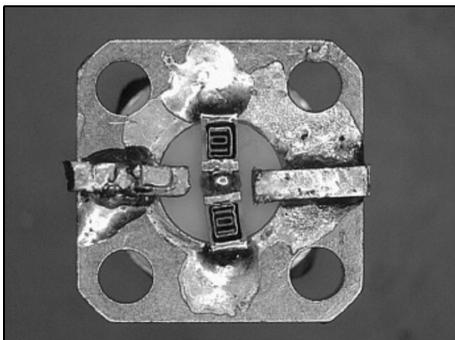
**Fig 13: Homemade 50Ω load.**
