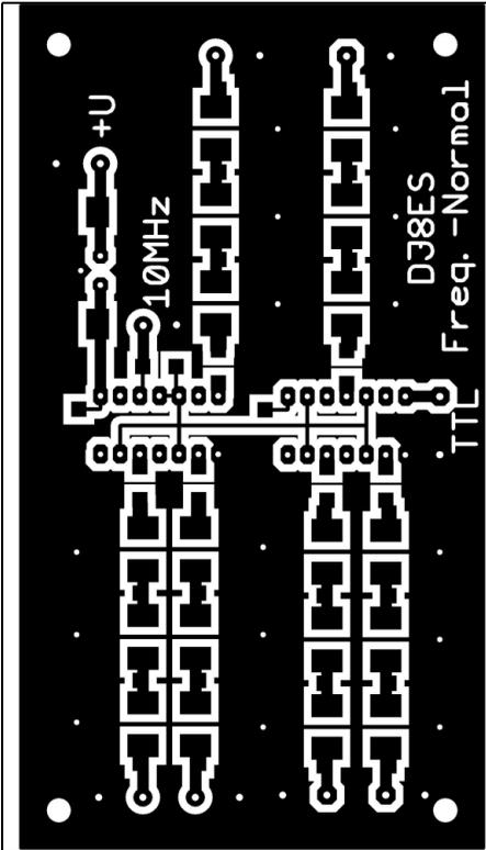
**Fig 9: The layout for the top side of the six 10MHz output PCB.**
