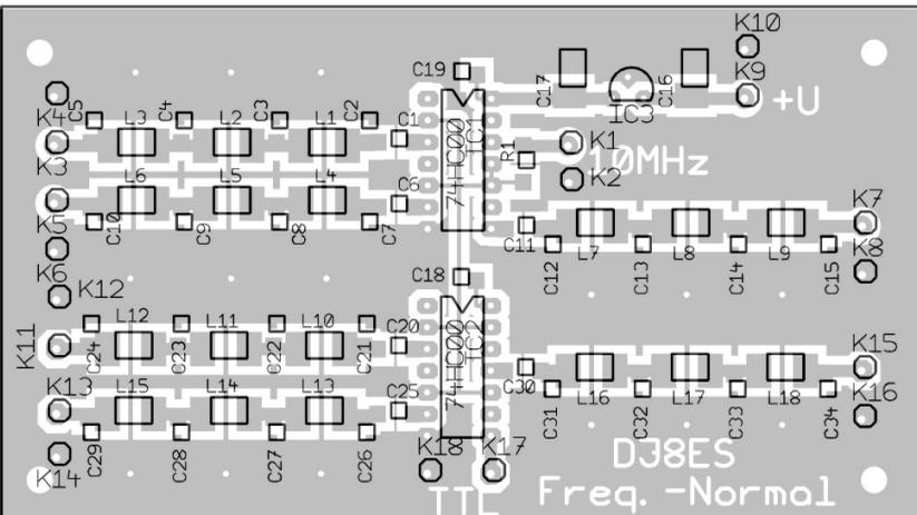
**Fig 11: The component layout for the six 10MHz output PCB.**
