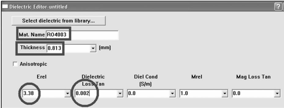
**Fig 11: The characteristics of the PCB material (Rogers RO4003) must be registered accurately. See text.**
