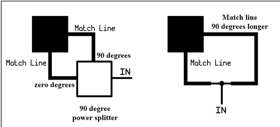
**Fig 3: The two possibilities to produce circular polarisation with a square patch antenna.**
