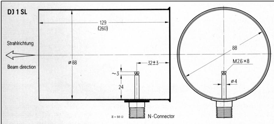
**Fig 3: Dimensions of a tubular radiator for the 13cm band.**
