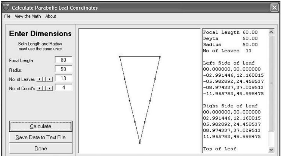
Fig 6: Parabola Leaf calculator results screen.
