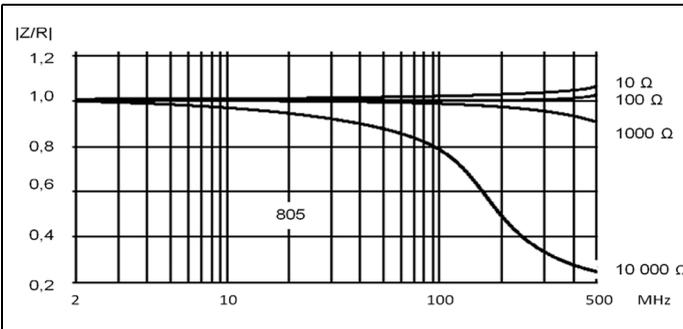
**Fig 8: Example of SMD thin layer 0805 behaviour vs. frequency.**
