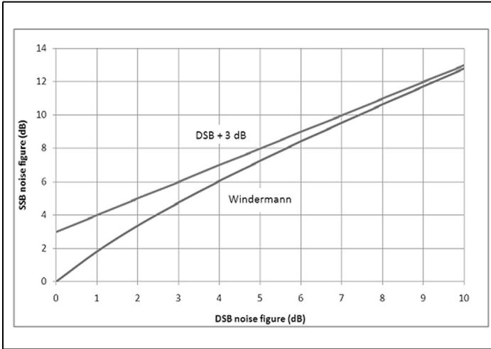
**Fig 6: True SSB figure and DSB +3dB versus DSB figure.**
