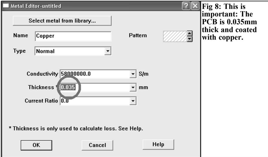
copper layer is set to  $35\mu\text{m} = 0.035\text{mm}$  and confirmed by pressing OK. The overview menu ensures that everything drawn later is realised in copper (Fig 9).
