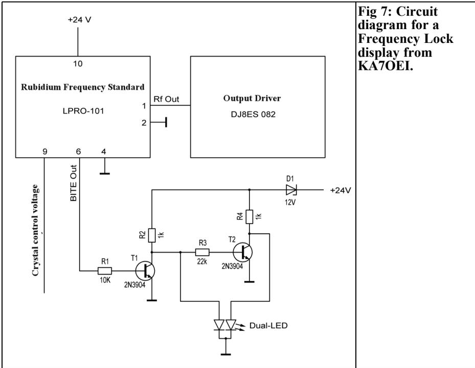
**Fig 7: Circuit diagram for a Frequency Lock display from KA7OEI.**
