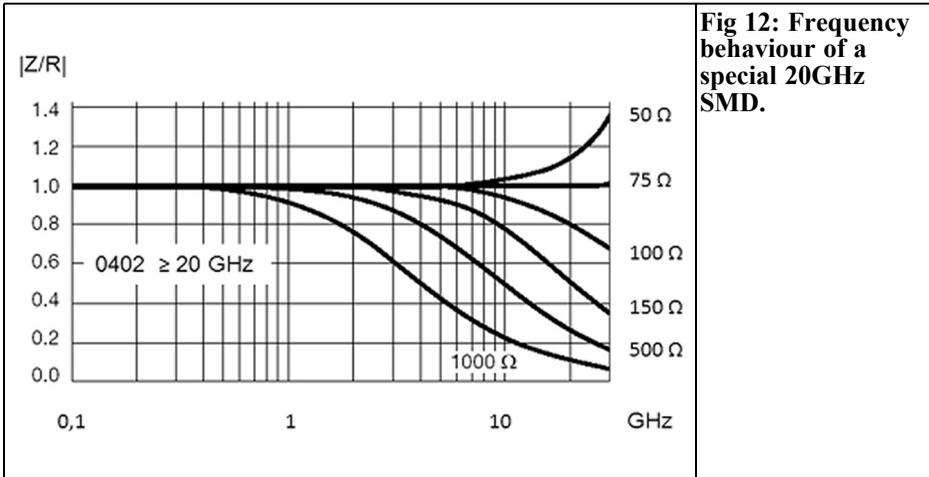
ROS is 1.15 to 10GHz. Tests with a single 50Ω or three 150Ω in parallel have given worse results.
