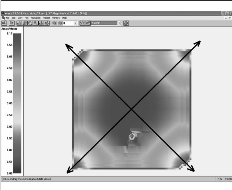
**Fig 21:** The current distribution at the required centre frequency is fascinating. It is easy to see the two active antennas, even in black and white. It looks much better in colour - Andy.
