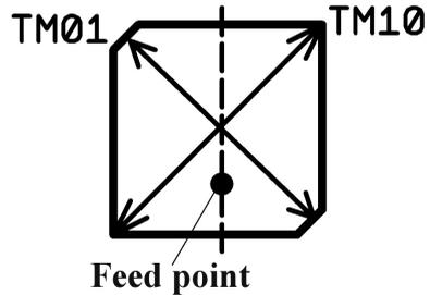
**Fig 6: Third and most popular possibility: the corners are cut at 45 degrees, otherwise the same as Fig 5.**
