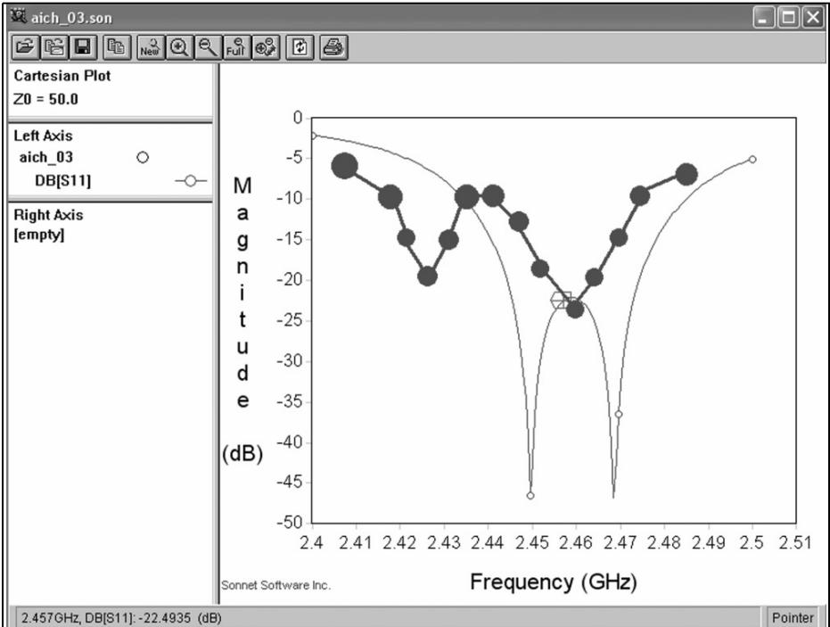
**Fig 20:** That is the difference between theory and practice! The result is 10MHz below the required centre frequency of 2.45GHz.
