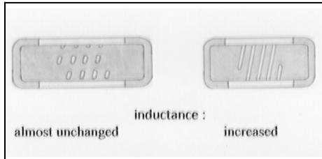
**Fig 11: Trimming of cylindrical resistor by sanding or laser.**
