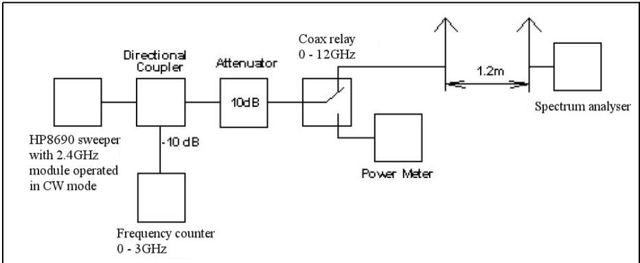
**Fig 22: This is the measurement setup (here for 2.45GHz) that has been used successfully several times to perform gain measurements on antennas in the far field. See text.**
