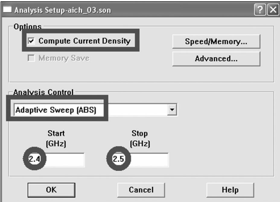
Fig 16: The last job before starting the simulation is to programme the sweeps.
