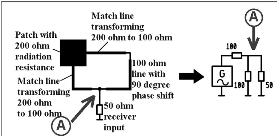
**Fig 24:** The equivalent circuit produced from the antenna on the left makes it possible to understand the behaviour of the antenna. See text.
