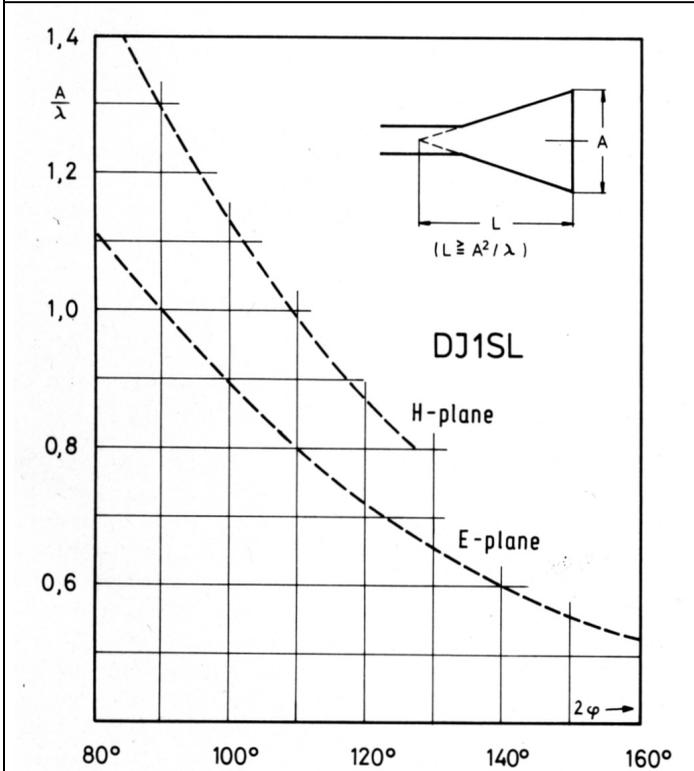
Fig 2: 10dB beamwidth  $2\phi$  of horn radiators.
