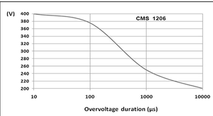
**Fig 3: Example of maximum permissible peak pulse voltage as a function of its duration.**
