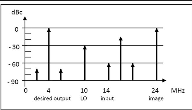
**Fig 3: Sample of a mixer output.**
