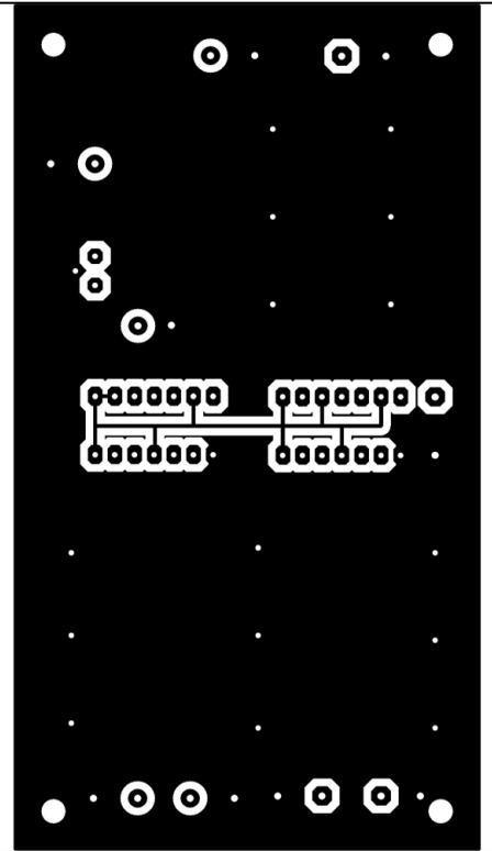
**Fig 10: The layout for the bottom side of the six 10MHz output PCB.**
