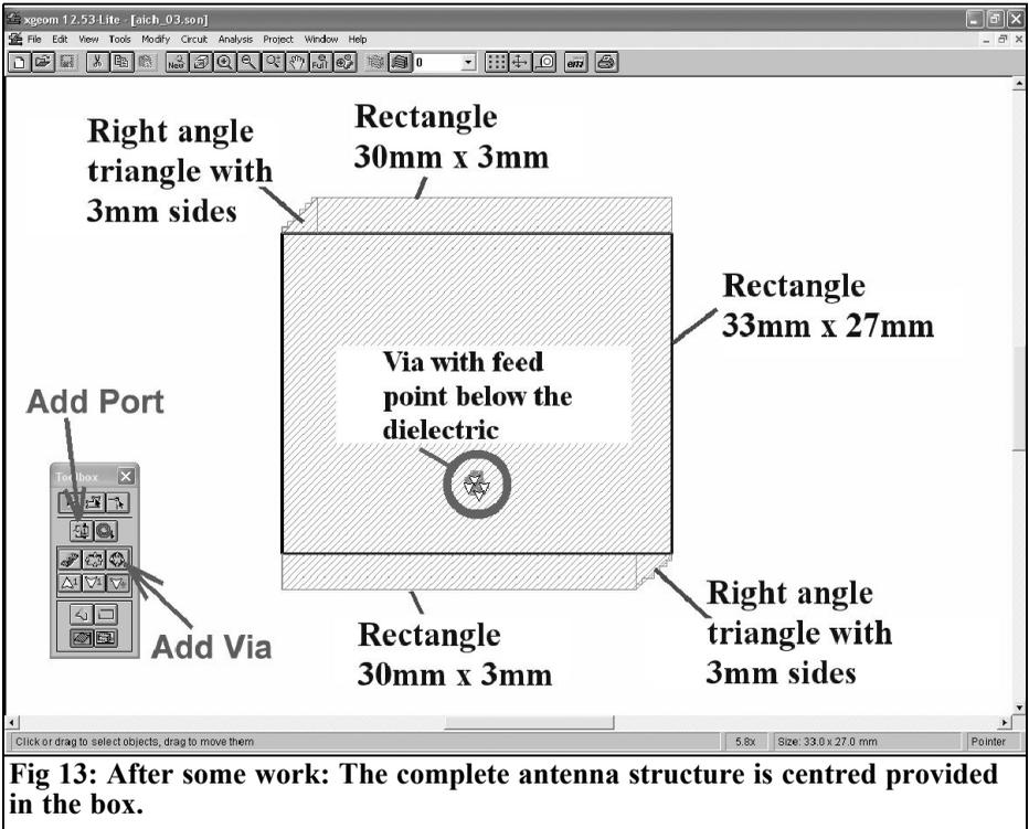
**Fig 13: After some work: The complete antenna structure is centred provided in the box.**
