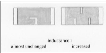
**Fig 10: Chip resistor trimming.**
