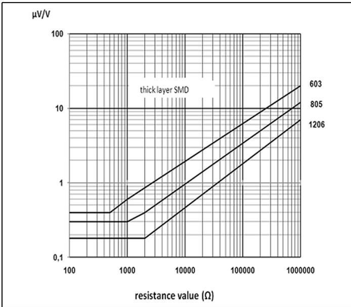
**Fig 6: Excess noise of SMD thick layer resistor.**
