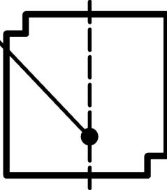
**Fig 5: Second possibility: the patch is square with the corners punched out, the feed point is on the centre line.**
