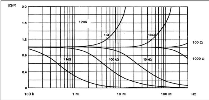
**Fig 9: Example of SMD thick layer 1206 behaviour vs. frequency.**
