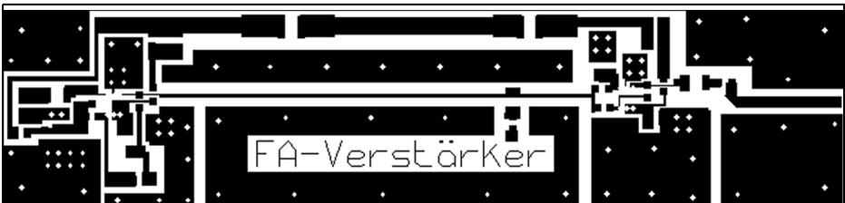
**Fig 10:** The PCB layout shows the additions needed for a high gain amplifier in a small space. (see text).
